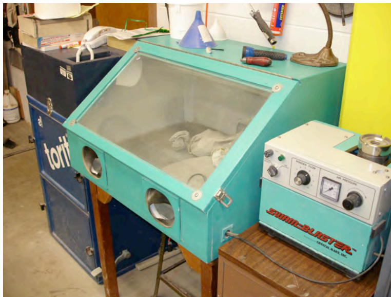
Figure 10. The Swam Blaster air abrasive unit and its dedicated Torit dust collector.
