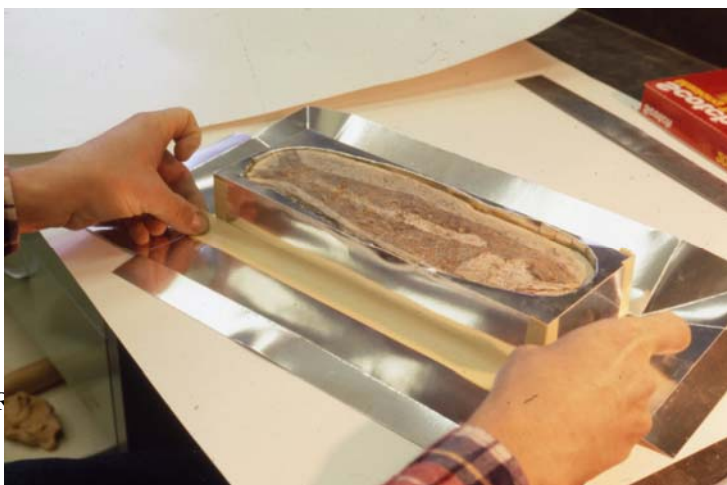
Securing the inner box to the outer box using masking tape. The pieces of masking tape must be long enough to seal the edge of the inner box to the outer box.
