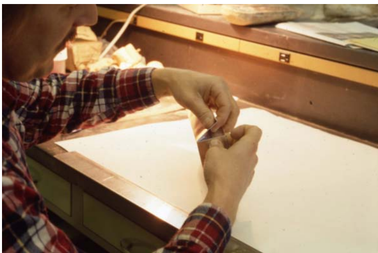
Folding the corners on the inner box. The corners get folded inward on the inner box.
