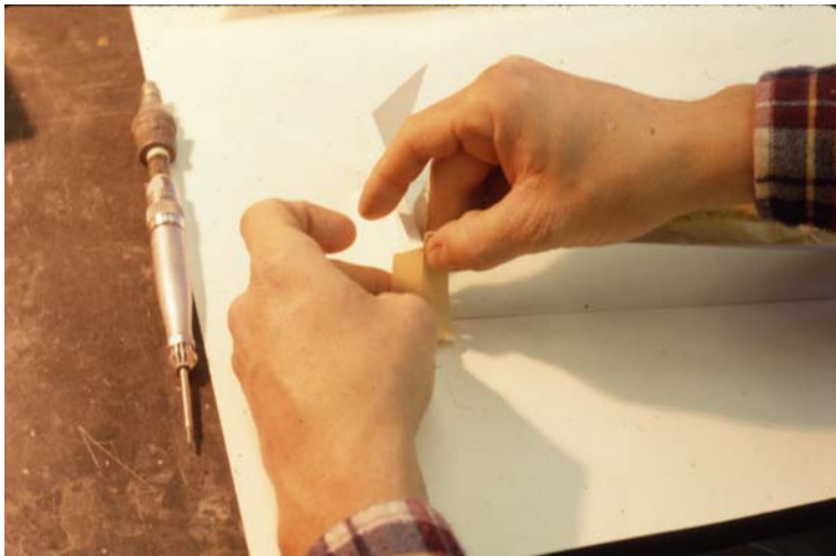
Sealing the corners of the inner box with masking tape.
