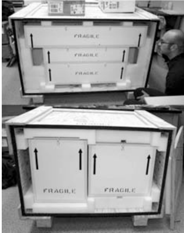
Figure 6: Foamcore boxes secured within the crates.
