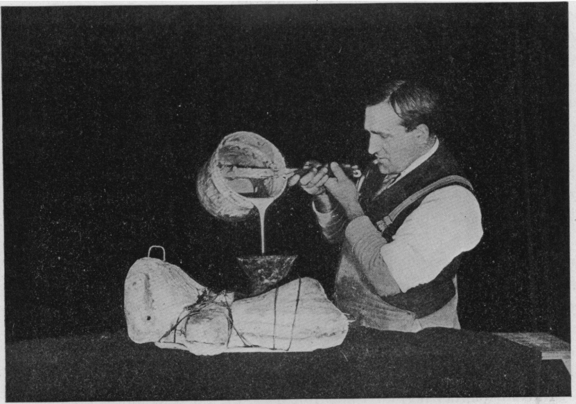
Fig. 7. Pouring gelatine into mould.
