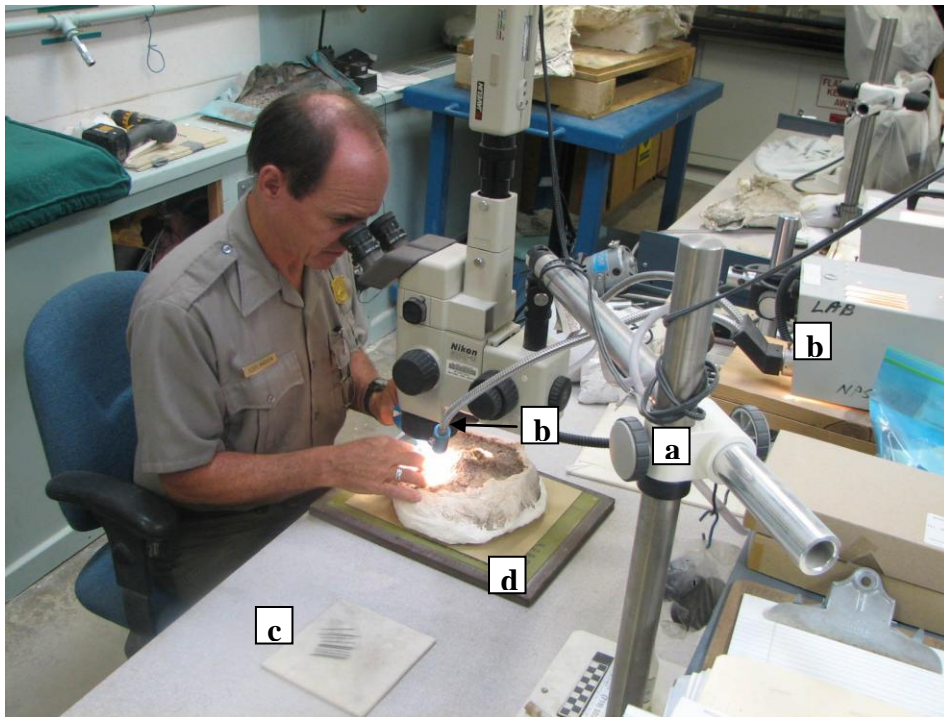
Figure 1. My work set-up at Dinosaur National Monument. Notice the following equipment: sturdy table, comfy adjustable chair, adjustable boom stand (a), fiber optic light (b), selection of sharpened carbide needles (c), and moveable work surface (d). The air line is not readily visible in the wires coiled on the boom stand. Also notice the relaxed shoulders and neck, a result of correct work surface and eye-piece heights.
