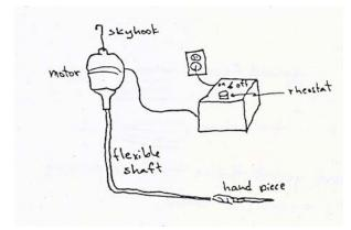
fossil preparation, by far the most useful one I have come across is the Ernst Baehr tool. It consists of a hanging variable speed motor with flexible shaft and interchangeable hand pieces. It comes with a foot-pedal rheostat, but I prefer a hand rheostat, which is easier to maintain a constant speed. I have mine hooked up with an on-off switch in series with the rheostat.
