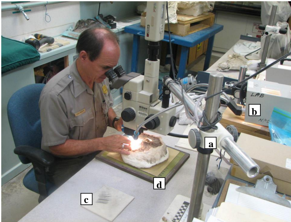
Figure 1. My work setup at Dinosaur National Monument. Notice the following equipment: sturdy table, comfy adjustable chair, adjustable boom stand (a), fiber optic light (b), selection of sharpened carbide needles (c), and moveable work surface (d). The air line is not readily visible in the wires coiled on the boom stand. Also notice the relaxed shoulders and neck, a result of correct work surface and eye-piece heights.
